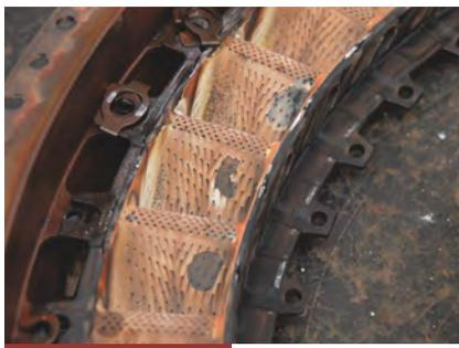
**HOT-SECTION VANE** as removed from the engine.
